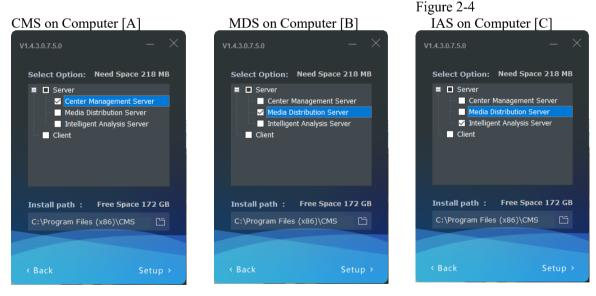
After the CMS server is installed, you need to use the server management tool to configure the IP of the central management server, the media distribution server and the intelligent analysis server, which are all managed by the central management server. The CMS management tool is automatically displayed in the system tray after the system is installed. After displaying the main interface, select the corresponding service and click "Configure", as shown in figure 2-5.
