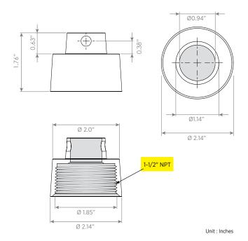
1-1/2 NPT is not compatible with G 1-1/2" threads. Verify camera/device manufacturer specifications.
