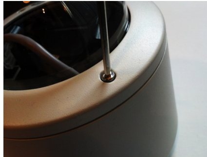
(b) Remove screws
