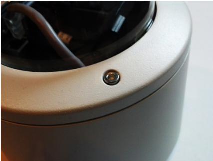
(a) Locate vandal screws
