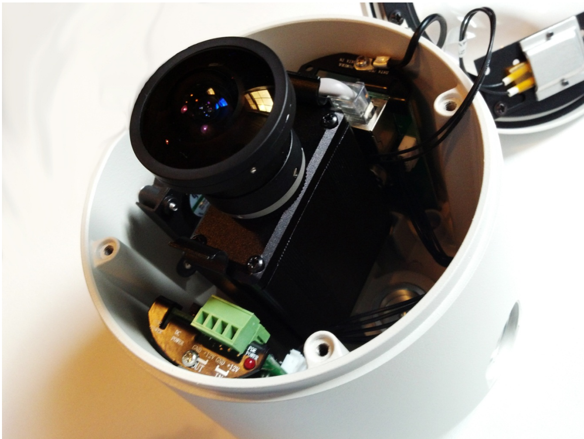
Finished installation of camera into dome housing.
