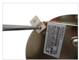
5. Align and insert the camera base hooks to the mounting holes of the metal plate.
