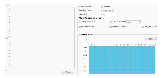
**2.** Select **Enable** for **Audio Detection**, select a detection type and set the difference or threshold. To disable audio detection, clear the **Enable** check box.
