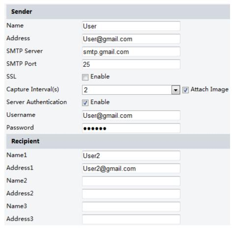
2. Configure relevant parameters of the sender and the recipient
