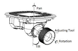
9. Tighten the hex screw to fix the well-adjusted surveillance angle.
