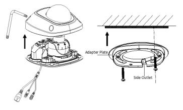
8. Use the supplied adjusting tool to adjust the pan  $[\pm 30^{\circ}]$ , tilt  $[0 \sim 80^{\circ}]$ , and rotation direction  $[0 \sim 360^{\circ}]$ .
