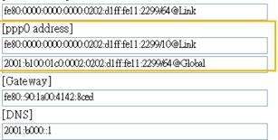
Manually setup the IP address: Select this option to manually set up IPv6 settings if your network environment does not have DHCPv6 server and advertisements-enabled routers.
