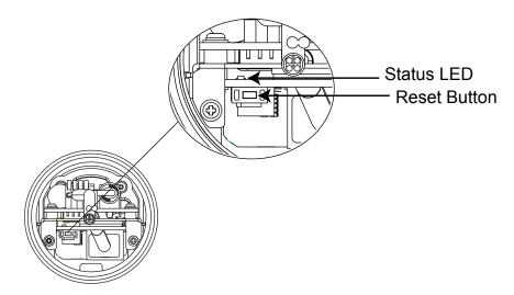
The reset button is used to reset the system or restore the factory default settings. Sometimes resetting the system can return the camera to normal operation. If the system problems remain after reset, restore the factory settings and install again.
