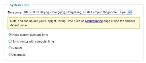
Keep current date and time: Select this option to preserve the current date and time of the Network Camera. The Network Camera's internal real-time clock maintains the date and time even when the power of the system is turned off.
