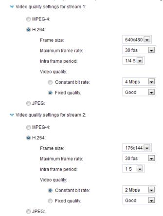
If H.264 / MPEG-4 mode is selected, the video is streamed via RTSP protocol. There are four parameters for you to adjust the video performance:
