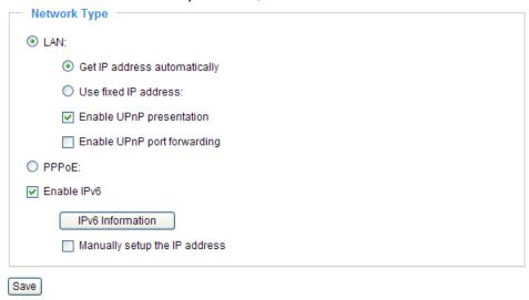
When IPv6 is enabled, by default, the network camera will listen to router advertisements and be assigned with a link-local IPv6 address accordingly.
